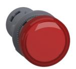
Monolithic pilot light, Easy Harmony XA2, plastic, red, 22mm, integral LED, screw clamp terminals, 24V AC DC
